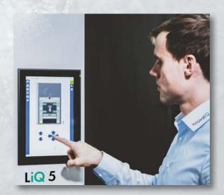
Our CNC-based control "GestiQPro" comes with a 12-inch touchscreen. The operator has all functions and parameters in scope. Users can easily interact with the system via the user-friendly control panel.
